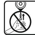
Do not release the device cable suddenly when extended
