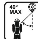
Permissible inclination of work line from the vertical line
